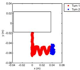
Figure 9: FT beam completely lost during a fully asynchronous beam dump on TIDVG in 2 turns.
