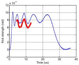
Figure 4: Kick strength seen by the tracked protons of the LHC beam (red) when all kicker firing. Kicker waveform (blue) for comparison.
