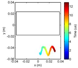
Figure 3: Protons of the LHC beam lost on the TIDVG front surface as a function of time within the beam (colorcoded), when all kickers are firing. Rectangle indicates aperture for circulating beam.
