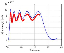
Figure 7: Kick strength seen by the FT beam shifted backwards by  $0.4 \,\mu s$  in relation to the kicker waveform.
