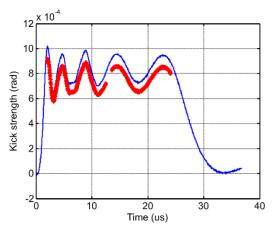
Figure 6: Kick strength seen by the FT beam in relation to the total kicker waveform.
