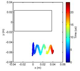
Figure 5: FT beam lost on the TIDVG front surface, when all kickers are firing.
