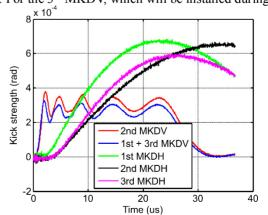
Figure 2: Waveforms of the vertical (MKDV) and horizontal kickers (MKDH) used for the simulation.
