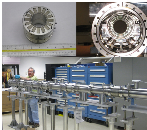
Figure 17: The design of the SNS BTF FODO beam line. The quadrupole permanent magnet is on top left, the magnet mounting structure is on top right, the assembled FODO line is at the bottom of the figure.
