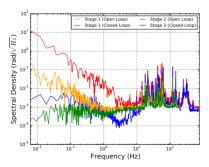
Figure 6: Noise spectrum of the cavity phase.
