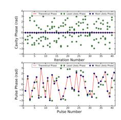
Figure 2: Cavity and pulse phases in direct iteration algobe used rithm.
