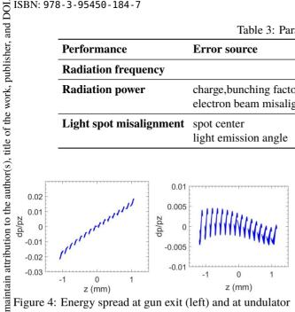
Figure 4: Energy spread at gun exit (left) and at undulator entrance (right).
