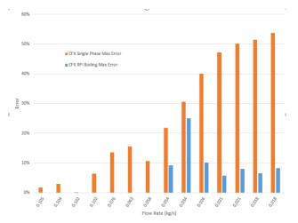
Figure 8: Maximum % difference found between CFX simulations and experimental validation of converter fins with RPI boiling model off and on.
