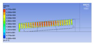
Figure 3: Cross-section through the horizontal plane along the beam axis showing flow balance in water between all fins.
