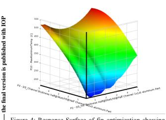
Figure 4: Response Surface of fin optimization showing temperature as a function of fin thickness and channel thickness.
