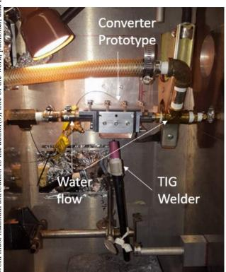
Figure 6: Validation testing apparatus.
