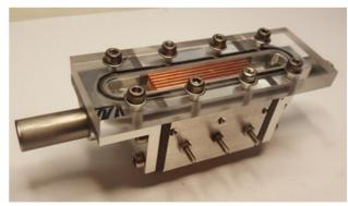
Figure 5: Prototype converter in housing; converter fins are copper surrounded by aluminum housing and a clear polycarbonate lid. Graphite thermally isolates the converter. Heat is applied to the bottom (not visible).
