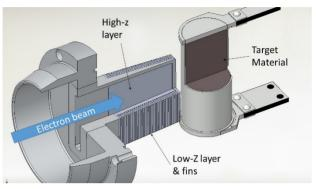
Figure 1: Layout of the converter and photofission target.
