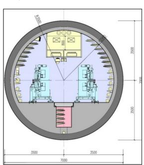
Figure 1: Cross section of undulator tunnel of SCLF.
