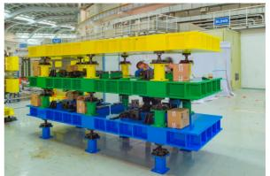
Figure 5: Three frames of stackable horizontal gap undulator.
