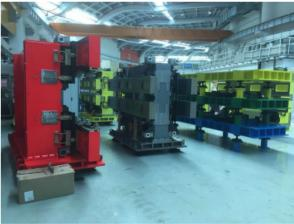
Figure 6: Three kinds of undulator are showing here, red one is a conventional undulator, two-in-one type undulator is in the middle(unpainted) and multi-color stackable undulator frame.
