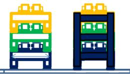
Figure 3: Layout of multi-layer horizontal gap undulators, Left, Stackable type; Right, One-frame type.
