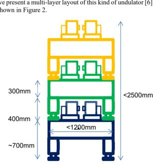
Figure 2: Scheme of stackable horizontal gap undulator.
