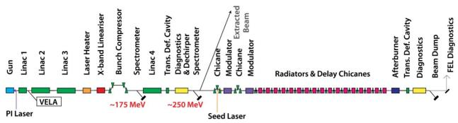
Figure 1: Schematic layout of CLARA. The total length is ~90 m.
