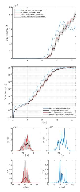
Figure 3: FEL simulation results. Top and second from top: FEL pulse energy with distance through the undulator on linear and log scales. Below: temporal profiles and spectra at saturation (15 m). For each plot there are multiple shot noise realisations shown for the Genesis results (grey), with one typical case highlighted (red) and the average also shown (black). One shot noise realisation is shown for Puffin (blue).
