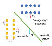
Figure 1: Simplified schematics of the "line" electron beamlet arrangement with spacing d.
