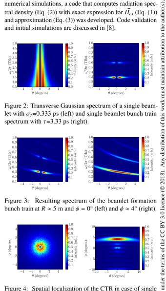
Figure 3: Resulting spectrum of the beamlet formation bunch train at  $R \approx 5$  m and  $\phi = 0^{\circ}$  (left) and  $\phi \approx 4^{\circ}$  (right).
