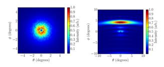
Figure 4: Spatial localization of the CTR in case of single Gaussian beamlet (left) and the extened CTR source formed by the beamlet bunch train (right) at the first harmonic frequency of  $\omega/2\pi=333$  GHz.
