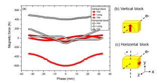
Figure 6: (a) Force calculations for two types of magnet blocks in various phases, where vertical blocks are marked (solid) and horizontal blocks (open) and for horizontal (square), longitudinal (circle) and vertical (triangle) force components. Two types of block rotation, vertical (b) and horizontal (c) along the axis are shown by the dashed arrow. The solid arrow indicates the magnetization direction.
