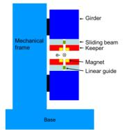
Figure 1: A typical structure of an APPLE-II undulator.
