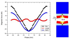
Figure 4: Magnetic force calculation of one array for various phases and horizontal (square), longitudinal (circle) and vertical (triangle) force components. The sketch shows the deformations of the four arrays schematically.
