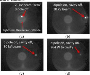
Figure 6: Beam images from in-line screen under various conditions.
