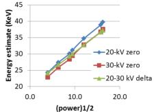
Figure 7: Beam kinetic energy vs RF input power using a 20-kV calibration (blue line), a 30-kV zero calibration (red line) and a third calibration using the power required to move the beam between the 20-kV and 30-kV calibration positions, for a fixed dipole field (green line).
