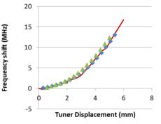
Figure 4: Cavity frequency shift vs. tuner position for two separate sweeps of the tuner (blue and green points) versus CST simulation results (red line).
