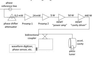
maintain attribution to the author(s), title of the Figure 1: Conceptual RF drive circuit for a single accelerator cavity, based around HEMTs. Note the lack of circumust lator between "cavity driver" HEMT and cavity.
