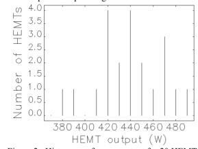
Figure 2: Histogram of power output for 20 HEMTs.
