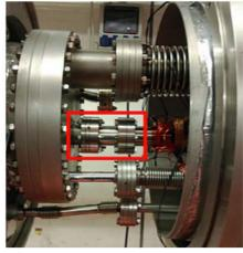
interconnection in between two modules is shown [11]. The big bellow of the helium gas return line is relatively stiff and can induce stress in between helium vessels from different modules. The beam tube is located in the red box.
