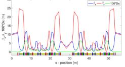
Figure 1: Optical functions and lattice structure for one cell of the HEPS storage ring.
