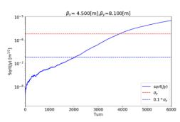
Figure 3: Maximum vertical amplitude of bunches with respect to number of turns for high brightness mode.
