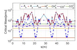
Figure 2: Calculated critical mass along the ring.
