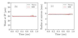
Figure 2: (a) SRW simulations of the amplification factor when phase correction procedure (feedback) is turned on and off. Results from a theoretical model are also shown. The seeding laser is turned off at  $t \approx 0.85$  ms. (b) SRW simulation of the spot size at cavity center with phase correction procedure turned on. Expected value is also shown. (c) The same for the spot size at either of the two mirrors.
