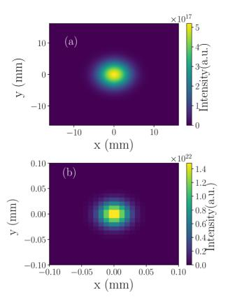
Figure 3: (a) SRW simulation of laser pulse transverse projection image at the first mirror. (b) Same for the spot at beam waist located at the center of the cavity.
