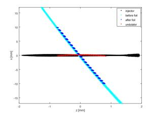
Figure 2: Transverse profile of the electron beam as a function of the longitudinal coordinate with a 4 THz prebunching at different locations along the terahertz facility.
