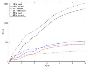
Figure 4: Energy of the the created radiation along the undulator for different wavelengths.
