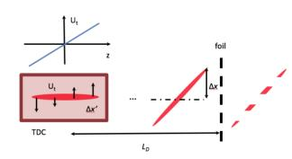
Figure 1: Pre-bunching scheme using a slotted-foil in combination with a transverse deflecting cavity.
