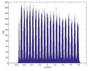
Figure 3: Current profile of the electron beam at the entrance of the undulator with a 4 THz pre-bunching.
