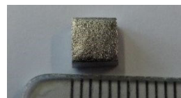
Figure 1: Niobium test samples cut from high quality Nb sheet. Typical sample size was 5x5x2.7 mm 3 . Distance between two marks is 1 mm.
