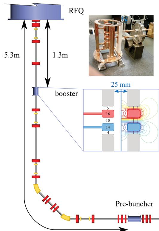
Figure 1: Pre-buncher, booster (inlay photo) and RFQ location at ISAC-I.
