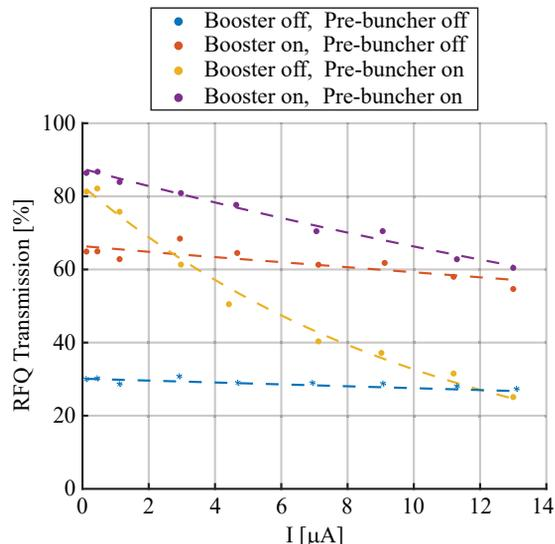
Figure 6: Booster operating as a buncher in different modes, as single or tandem with the pre-buncher, for  $^{20}\text{Ne}^{1+}$ .
