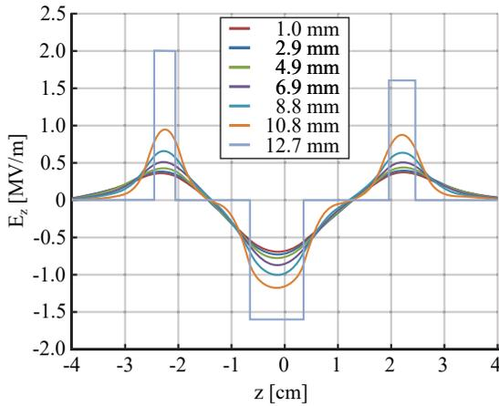
Figure 2: Accelerating field amplitude as a function of radius.
