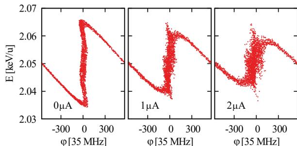
Figure 5: PARMELA simulated particle distribution including space charge effects for three different bunch charges and an  $A/Q = 30$  for 2000 particles. [5]
