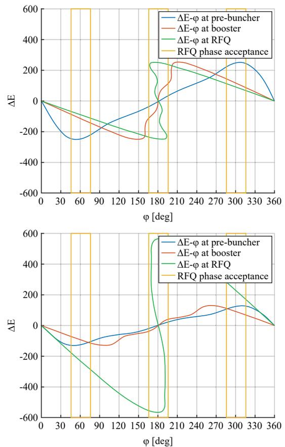
Figure 4: On top is the longitudinal phase space development for the multi-harmonic pre-buncher and at the bottom the longitudinal phase space development for tandem operation (pre-buncher and booster) is depicted for a  $^{16}\text{O}^{1+}$  ion beam at different positions in ISAC-I.
