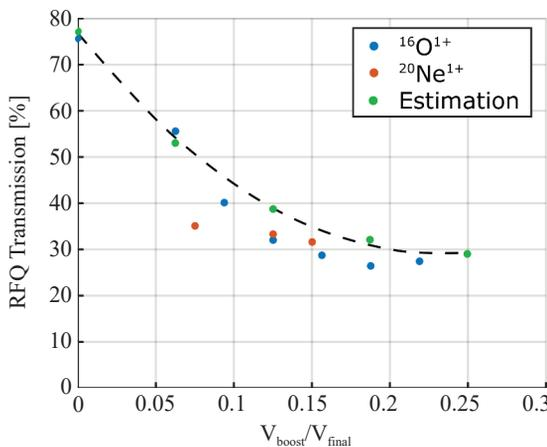
Figure 3: Measured RFQ transmission versus booster voltage, compared against expectation.
