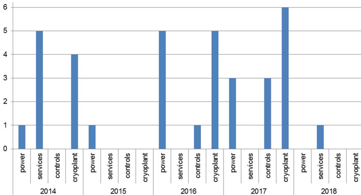
Figure 3: Interruptions of cryogenic system operation over 2014-2018 runs.
