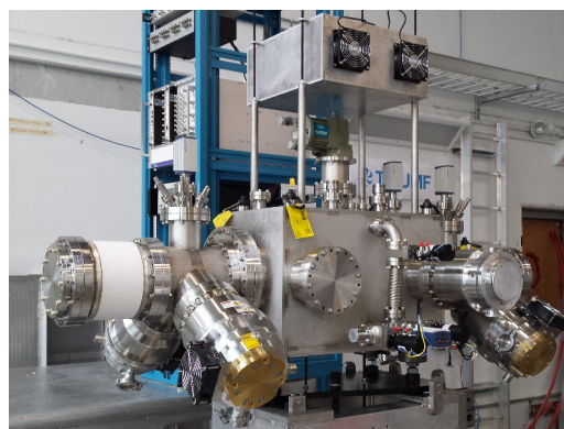
Figure 6: CANREB RFQ buncher installed in the ARIEL hall at TRIUMF.
