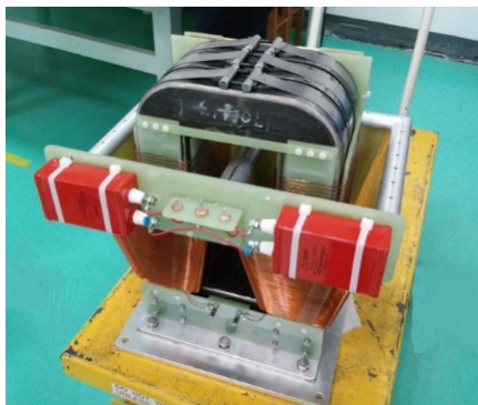
Figure 7: Picture of pulse transformer.
