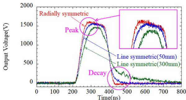
Figure 8: Measurement result of output waveforms when output voltage is doubled.
