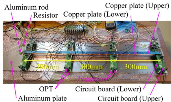
Figure 9: Test condition with a circuit distance of 300 mm and voltage doubled.
