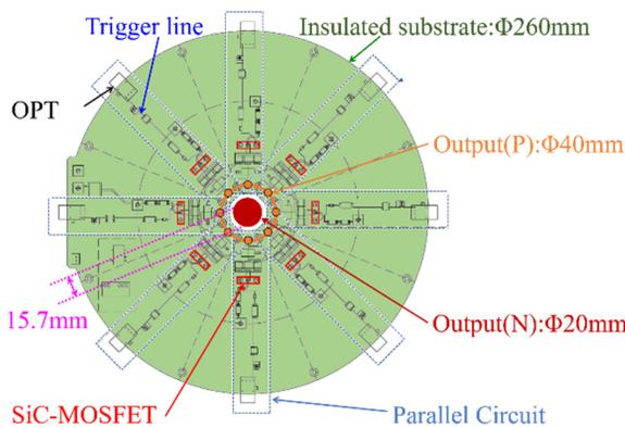
Figure 3: Schematic diagram of radially-symmetrical type base circuit.
