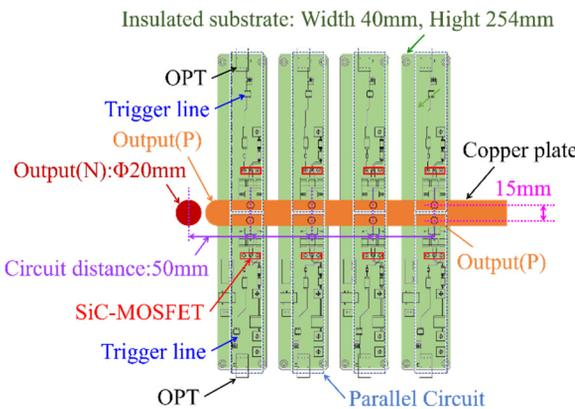
Figure 4: Schematic diagram of line-symmetrical type.
