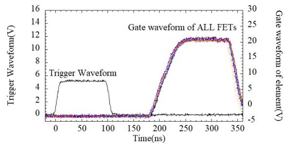
Figure 6: Measurements results of the gate waveform of all MOSFETs of each type.
