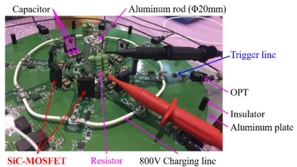
Figure 5: Situation of output voltage measurement using the radially-symmetrical type.
