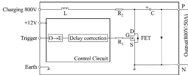
Figure 1: Block diagram of base circuit.
