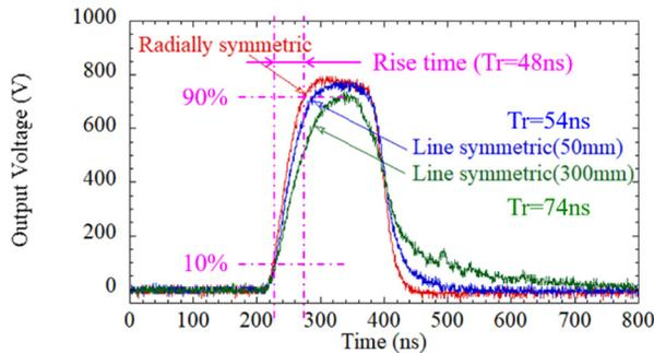
Figure 7: Measurement result of output waveforms by three symmetrical circuits.
