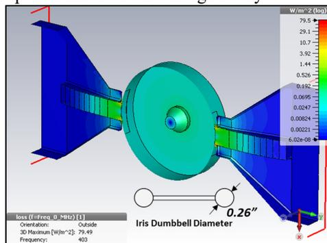
Figure 1: The surface power loss density of two iris couplers and a single cell cavity model for RF simulation. (blue is low  $6e-8$  W/m<sup>2</sup> and red high  $79.5$  W/m<sup>2</sup>)
