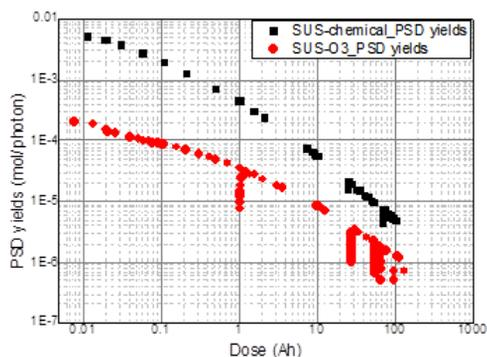
Figure 3: Photon stimulated desorption yields for different cleaning methods versus total beam dose.
