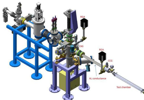
Figure 1: Experimental setup at the TLS beamline 19B.
