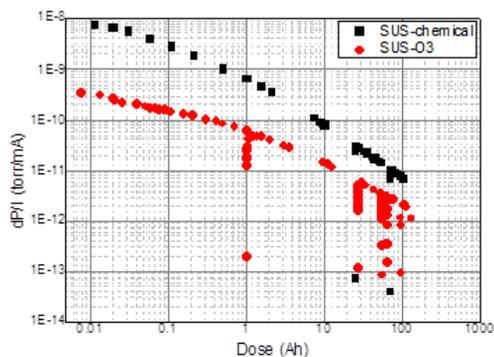
Figure 2: Beam current normalized vacuum pressure rise for different cleaning methods versus total beam dose.
