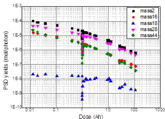
Figure 7: Photon stimulated desorption yields for different masses of ozonated water cleaned chamber versus total beam doses.
