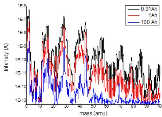
Figure 4: RGA spectrum for a chemically cleaned chamber at different beam doses.
