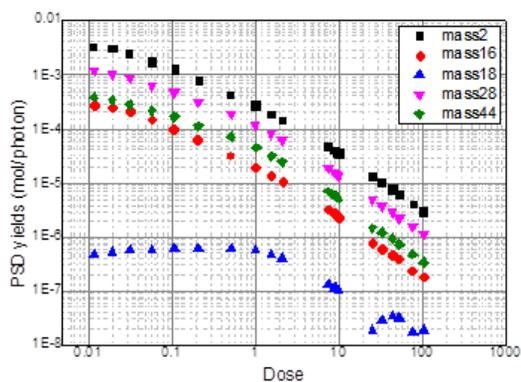
Figure 6: Photon stimulated desorption yields for different masses of chemically cleaned chamber versus total beam doses.
