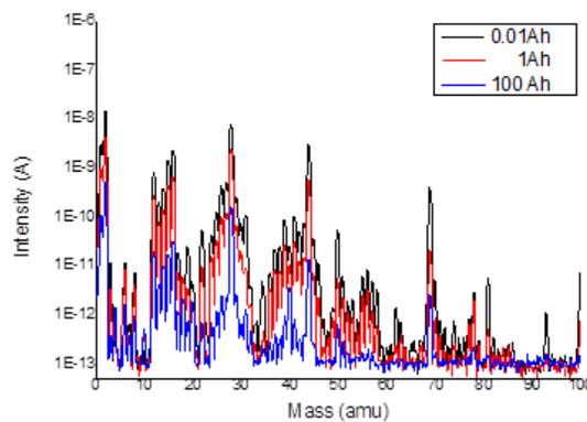
Figure 5: RGA spectrum after ozonated water cleaning of the chamber at different beam doses.
