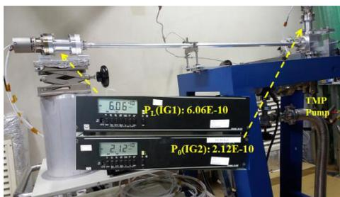
Figure 7: Photograph of the experimental system for the 1 m beam duct of AL(b).
