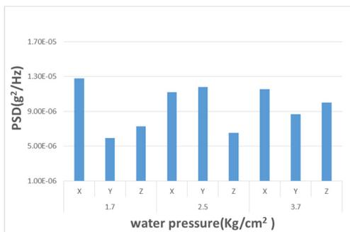
Figure 4: Vibration measurements for different water pressures.
