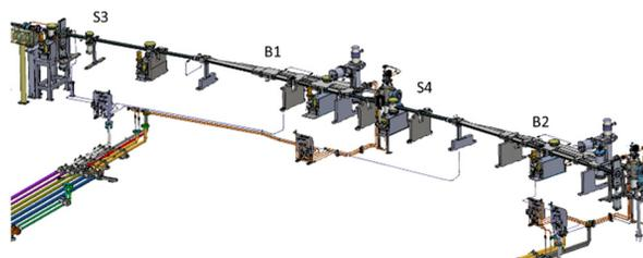
Figure 1: 3D drawing of one vacuum cell.
