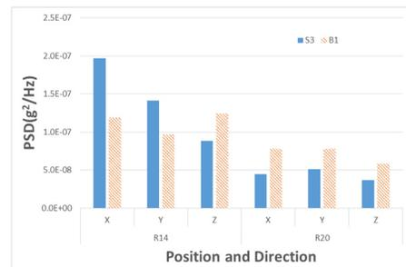
Figure 6: Comparison of vibration measurements between two different materials for the water tubes.
