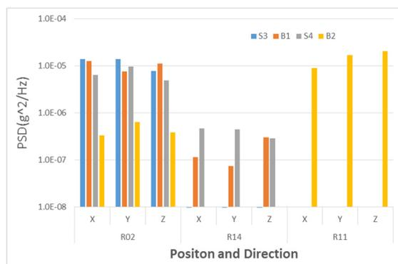
Figure 3: Vibration results under normal cooling water flow condition.
