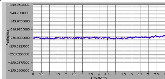
Figure 5(b): Output current waveform of the polarity reversal device when the polar switch is in the ON state.
