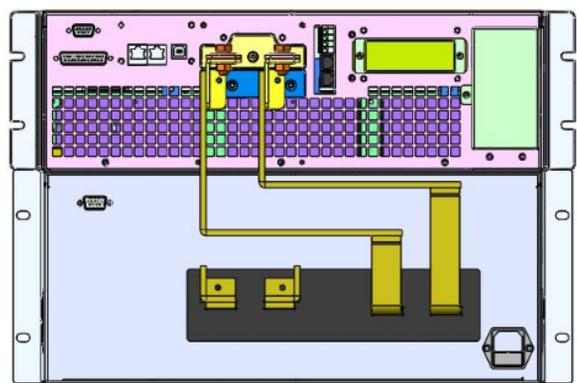
Figure 2: Diagram of the polarity reversal mechanism and DC source power supply.
