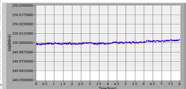
Figure 5(a): Output current waveform of the polarity reversal device when the polar switch is in the OFF state.
