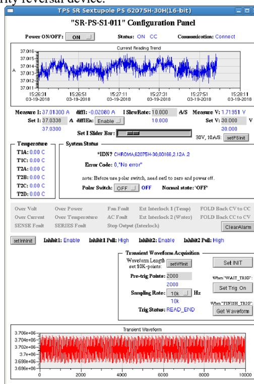
Figure 3: Remote control panel.
