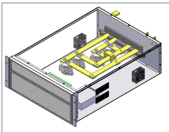
Figure 1: Diagram of the polarity reversal mechanism.
