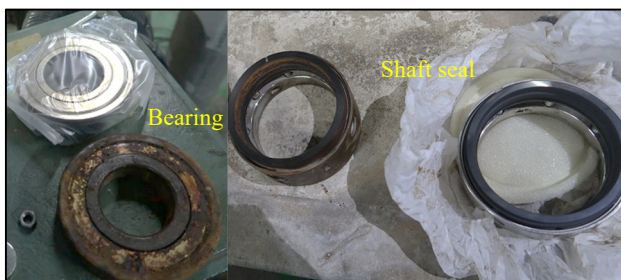
Figure 5: The original bearing and shaft seal and new ones for ZP6 pump system.
