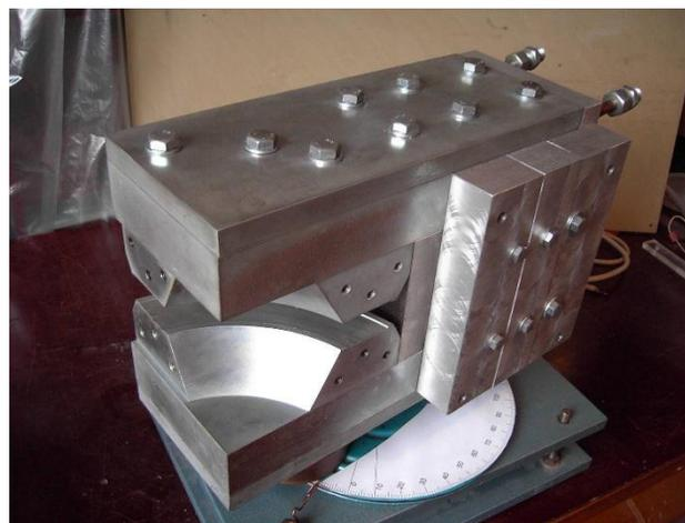
Figure 4: Dipole magnet for “EPOS” linear electron accelerator.
