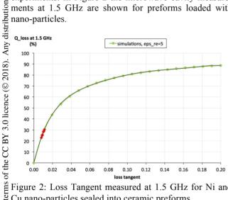
Figure 2: Loss Tangent measured at 1.5 GHz for Ni and Cu nano-particles sealed into ceramic preforms.
