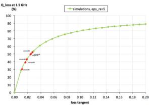
Figure 4: Loss Tangent measured at 1.5 GHz for Carbon sub-micron particles in ceramic preforms.
