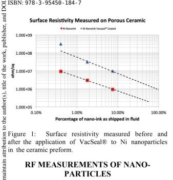
Figure 1: Surface resistivity measured before and after the application of VacSeal® to Ni nanoparticles in the ceramic preform.
