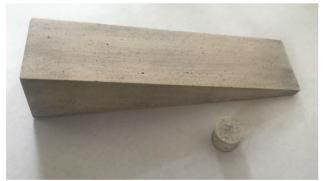
Figure 5: 90-92% dense ceramic with surface pores filled with sub-micron carbon particles.
