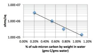
Figure 3: Surface resistivity as a function of the percentage by weight of carbon in water to form the slurry.
