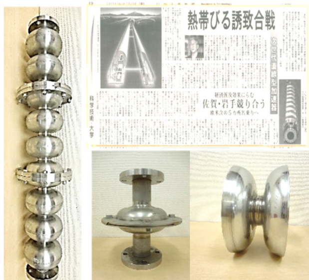
Figure 1: Photos of the newspaper article and stainless steel cavities (dumbbell, single cell, 9-cell).
