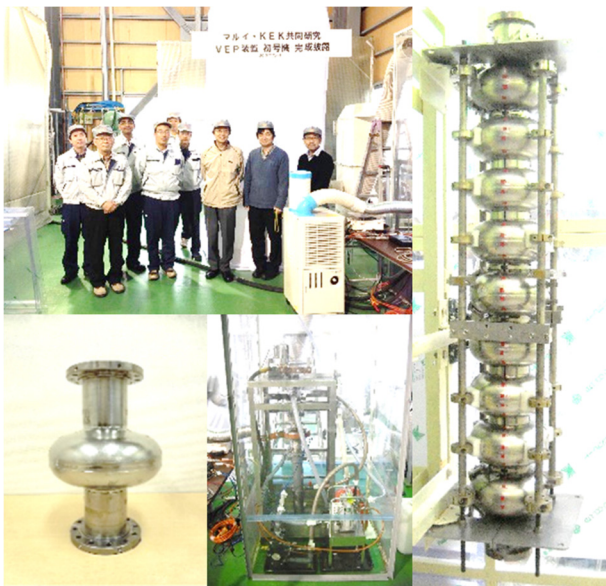
Figure 2: Photos of a niobium single cell cavity, a niobium 9-cell cavity, a first type VEP setup used for this confirmation, and Marui-KEK member.
