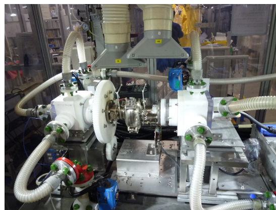
Figure 1: Single-cell coupon cavity on the HEP bed at KEK and a data logger attached to the cavity.
