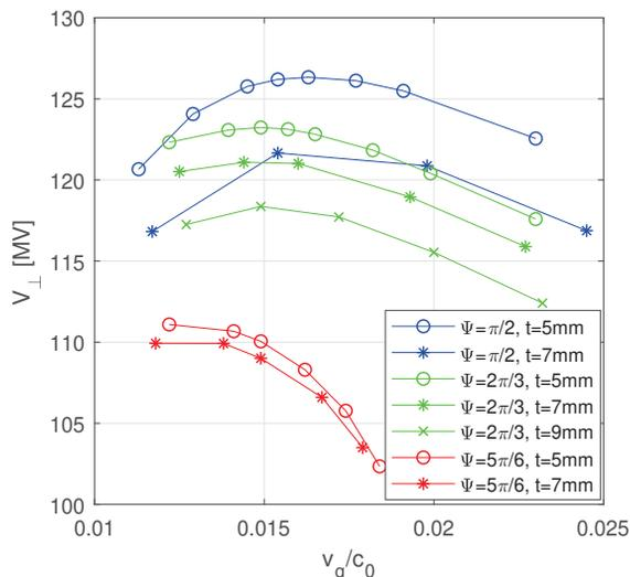
Figure 4: The total deflecting voltage for two structures with the RF set-up shown in Fig. 1.
