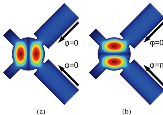
Figure 5:  $|E|$  in the coupler cell when deflecting the beam in the horizontal plane (a), and in the vertical plane (b). The two feeding waveguides are to the right, and the two matching stubs are to the left.  $\varphi$  is the relative phase of the incoming RF signal.
