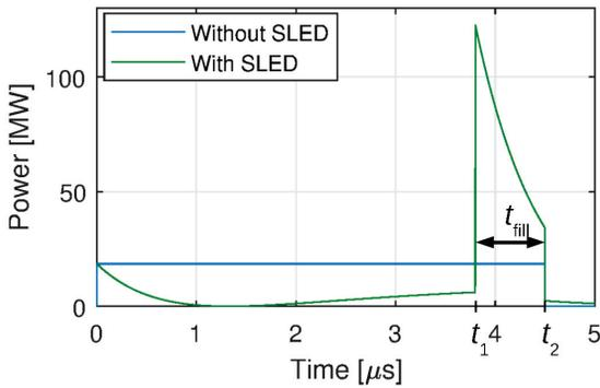
Figure 2: The maximum rms power delivered to one structure.
