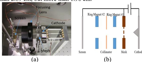
Figure 6: Photograph of current experimental setup (a) alongside a simple schematic of the setup (b).
