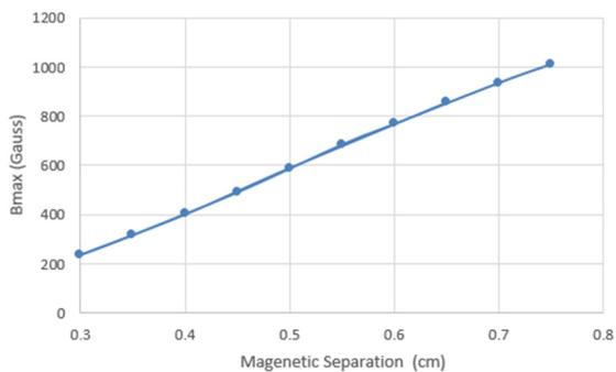
Figure 3: The relation between magnet separation and the peak on-axis field.
