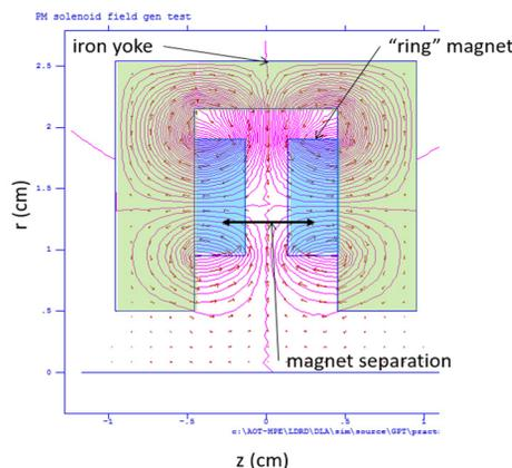
Figure 1: Poisson calculation of magnetic field of the lens. The lens consists of an outer iron yoke, and two inner ‘ring’ magnets which oppose each other.
