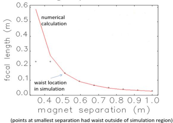
Figure 2: Comparison between on-axis predicted focal length, and particle tracking through a z-r field map.
