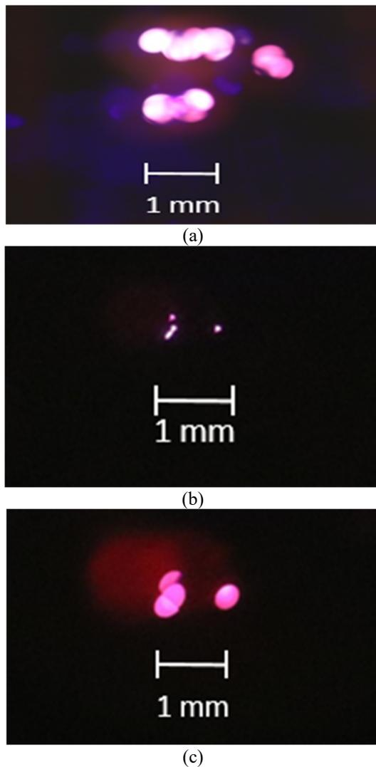
Figure 7: Comparison between an unfocused beam without a lens (a), our focused beam (b) at 23.5 mm, and our unfocused beam (c) at a distance of 30.5 mm. The focused beam has a spot size of 75  $\mu\text{m}$  while the unfocused beam measured at 197  $\mu\text{m}$
