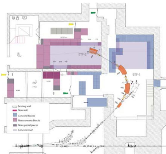
Figure 1: New configuration of the Transfer Line, the two BTF lines and the experimental hall.
