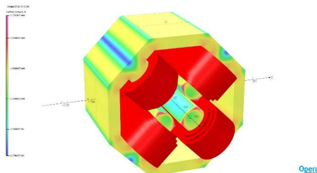
Figure 3: Schematic view of the quadrupole showing the saturation level.
