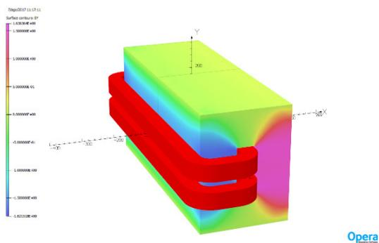
Figure 2: Schematic view of the DP01 magnet showing the saturation level.
