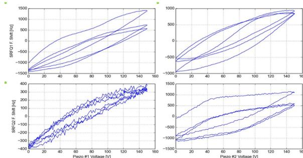
Figure 6: Tuning window of the Fast Tuners of SRFQ2 after the maintenance.
