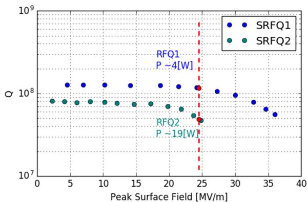
Figure 2: Q vs Em,s curves of SRFQ1 and SRFQ2 after the herein described special maintenance.
