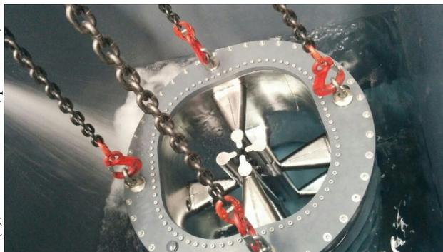
Figure 1: SRFQs during BCP at CERN.
