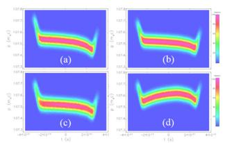
Figure 4: Longitudinal phase space at the exit of the simple arc simulating CSR with (a) elegant (b) GPT (c) GPT including space charge (d) Bmad including the effects of shielding from a 2" full aperture.
