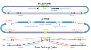
Figure 1: Schematic of the JLEIC bunched-beam electron cooler. The ERL (top) generates and transports beam to the CCR (middle) via a beam exchange region (bottom) where bunches make 11 recirculations before returning to the ERL for recovery.
