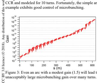
Figure 3: Even an arc with a modest gain (1.5) will lead to unacceptably large microbunching gain over many turns.
