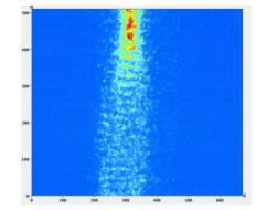
Figure 3. AWAKE milestone; first observation of proton beam self-modulation, reported in 2016. [8]
