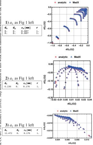
Figure 2: Sample IPs with r = 1: 1) head-on IP1 and 5; 2) single long range IP closest to IP5, bbip5L1 for half the nominal crossing angle (required  $q_{\text{max}}=25$ ); 3) same as 2),
