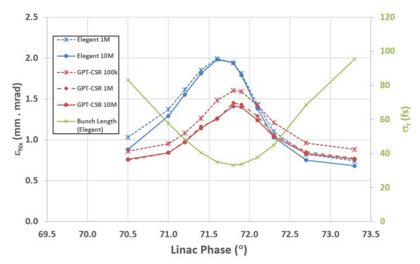
Figure 3: Example convergence study in Elegant and GPT-CSR for normalised emittance after the first bunch compressor of FERMI as a function of preceding linac phase. The energy at this position is 300 MeV, the bunch charge is 100 pC and the R<sub>56</sub> of the bunch compressor is fixed at 57 mm.
