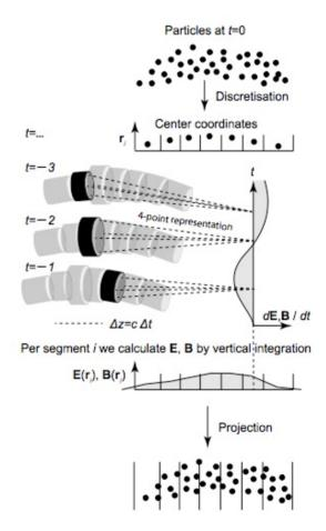
Figure 2: Schematic of field integration.
