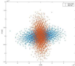
Figure 2: X-coordinate trace space for FBT with a 0.32 T field on the cathode.
