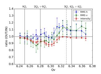
Figure 3: Ratios of final values (at 1285 ms) over initial values (at 185 ms) of the horizontal (blue) and vertical (green) RMS sizes of the bunch profiles and the intensity (red). Vertical lines indicate the relevant resonances (top).
