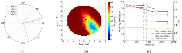
Figure 2: (a) RDT amplitude and phase for the skew sextupoles installed in the PS. (b) Scan of the currents of the "XSK14 and "XSK52" sextupoles with losses indicated by the color bar. (c) Intensity along the injection plateau corresponding to the natural excitation (no sextupoles) and the extreme cases of (b) together with the tune variation as a function of time.
