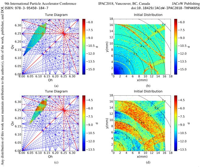
$\hat{\infty}$  Figure 4: FMA of on-momentum (a,b) and off-momentum (c,d) particles. Tune diagrams with resonances up to the 8<sup>th</sup>  $\widehat{S}$  order (a,c). The initial position of the particles tracked in the configuration space (b,d). The diffusion is used for the color © coding.
