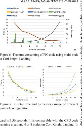
Figure 6: The time consuming of PIC code using multi-node at Cori knight Landing.
