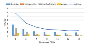
Figure 4: The scalability of the PIC code using  $64 \times 64 \times 64$ grid points and 1.6M particles on Titan.
