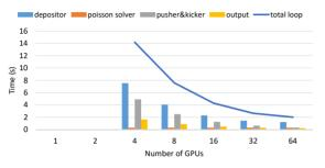
Figure 5: The scalability of the PIC code using  $64 \times 64 \times 64$ grid points and 16M particles on Titan.
