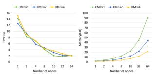
Figure 7: a) total time and b) memory usage of different parallel configuration.
