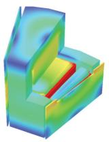
Figure 3: The input model of the main magnet in BOOSTER for the magnetic field calculation by TOSCA. Return yokes and field clamps are adopted.
