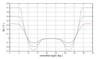
Figure 4:  $B_7$  vs  $\theta$  along different radii for the unit cell in BOOSTER. Red, green and blue lines correspond to radius of 1.2 m, 1.4 m and 1.6 m, respectively.
