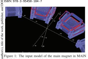
Figure 1: The input model of the main magnet in MAIN RING for the magnetic field calculation by TOSCA. Return RING for the magnetic field calculation by TOSCA. Return yokes are not installed to make energy variable beam ex-
