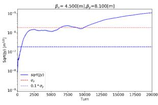
Figure 4: The evolution of the vertical oscillation amplitude of the beam with number of turns ( $n_b=63$ ).
