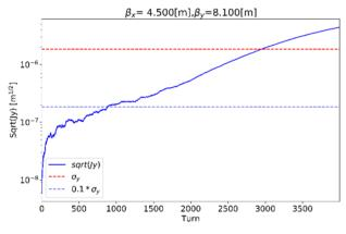
Figure 3: The evolution of the vertical oscillation amplitude of the beam with number of turns ( $n_b=680$ ).
