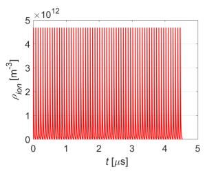
Figure 2: Ion density along the bunch train for the high charge mode ( $n_b=63$ ).
