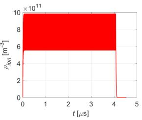
Figure 1: Ion density along the bunch train for the high brightness mode ( $n_b=680$ ).
