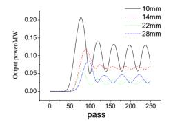
Figure 1: Output power as a function of the optical pass to different waveguide gap when the radiation frequency is 2THz.
