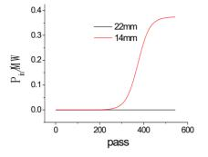
Figure 2: Resonator power as a function of the optical pass to waveguide gap 14mm and 22mm when the radiation frequency is 1THz.
