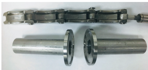
Figure 5: Chain clamp along with two flanges to form a cylindrical cavity for the experimental measurements.
