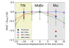
Figure 7: The measured difference in the real part of the Elongitudinal impedance suggests a higher than expected resistivity of the Mo stripe. Resonant wire measurement, performed in a test stand prior to the installation of the threestripe collimator in LHC.
