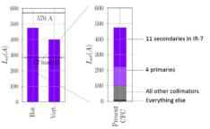
Figure 1: Impedance of LHC collimators is responsible for nearly all the octupole current needed to stabilize the beam, and has to be reduced to provide a stability margin for the Hi-Lumi upgrade [3]. BCMS beam, 7 TeV, beginning of the luminosity levelling process,  $\beta^{*}=41$  cm.
