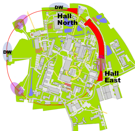
Figure 1: Layout of PETRA III with the location of damping wigglers (DW) and halls with a total of 24 beam lines.
