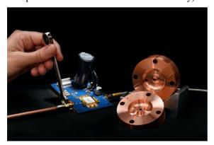
Figure 1: An HEMT with two halves of a copper cavity.
