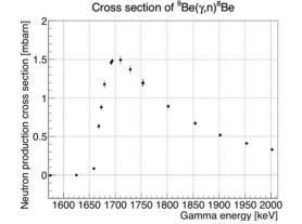
Figure 5: Photo-neutron production cross section of <sup>9</sup>Be [12]. The peak cross section is 1.5 mbarn at 1690 keV. Threshold energy is 1665 keV. This reaction produces monochromatic neutrons if  $\gamma$ -rays are monochromatic.
