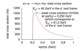
Figure 4: Total cross section of muon pair production in a fixed target.
