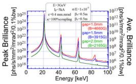
Figure 2: Example of the X-ray spectrum from veryshort-period undulator ( $\lambda u=4mm$ , L=1m) at ILC.
