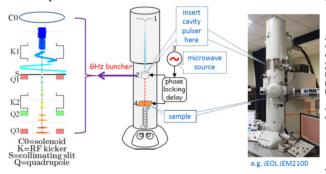
Figure 1: Basic principle of the stroboscopic laser-free high-duty cycle TEM: 1) DC electron source; 2) DC beam bunching device; 3) RF source; 4) the sample.
