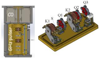
Figure 2: Engineering design of the entire unit, consisting of focusing C0 element and GHz buncher. All components are mounted on the vacuum compatible 3-axis translation stage.
